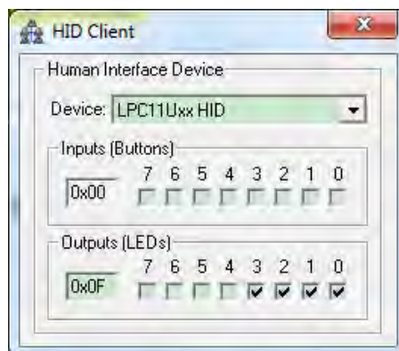
Fig 12. HID client utility (the HID device has been detected and selected)
